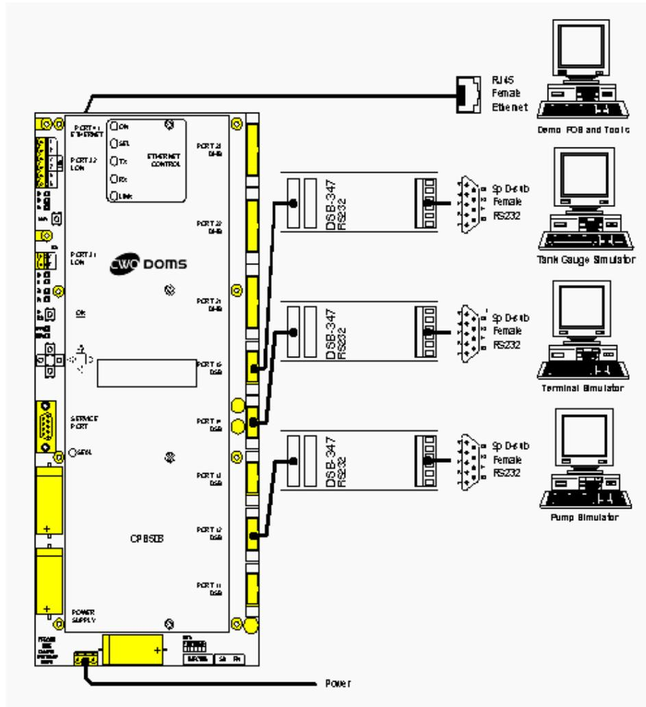
Fig. 1 Connecting TGSSim to the PSS 5000 System
